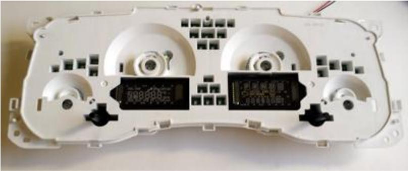
Install overlay, check for fit, install cover bezel to check alignment
