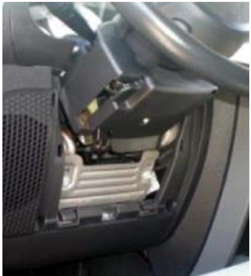
Remove the two bolts at the bottom of the cluster trim, lift off unit
