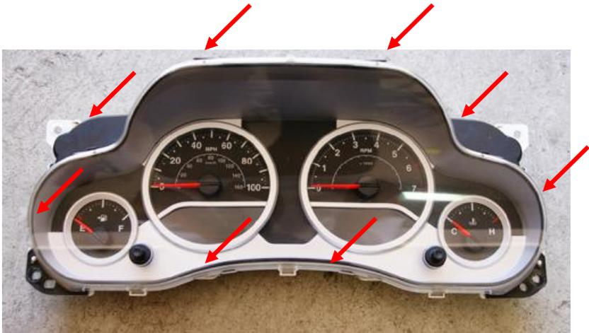
Lightly rotate pointers counter-clockwise until they hit the internal stops. Note the position by taking a photo or marking with tape
