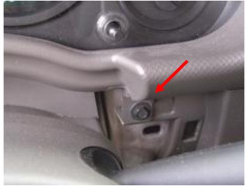
Cluster is held in place by 4 bolts, remove and pull cluster out enough to unplug all of the harnesses
