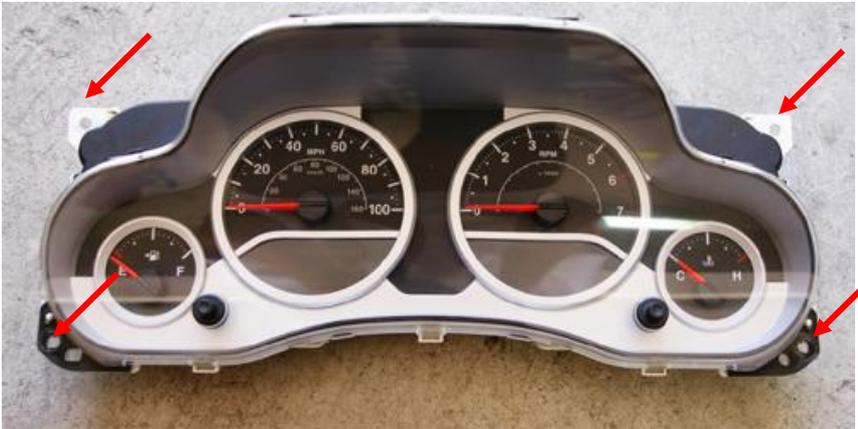
Press down on the tabs that secure the harnesses, remove plugs, there are four (4) of them.
