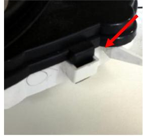
Unclip the eight (8) clips around the cover bezel and remove
