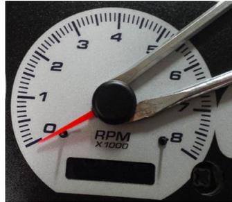
Remove the black plastic light blockers, just pry them off, retain for re-installation
