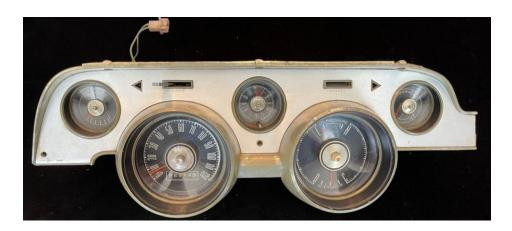
STEP 3: Remove the factory fasteners holding the factory instruments to the bezel. Remove all connectors and lights at this point
