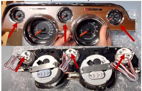
STEP 3.5: Connect 2" Jumper wires to the Speedo & Tach as shown below
