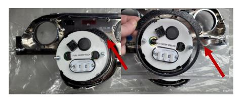
STEP 3.3: Place NVU bracket onto panel with the bulbs spacers towards the bezel
