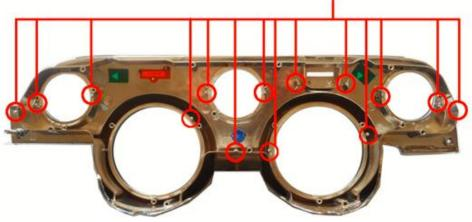
STEP 3.2: Now you have removed the standoffs, place gauges down into gauge holes(use 3 spacer rings per side)
