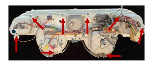
STEP 3.1: Now you have removed the Bezel, next Remove standoffs on bezel where indicated (use wire cutters)
