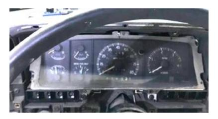
Remove the cluster retaining screws. Keep for re-use.
