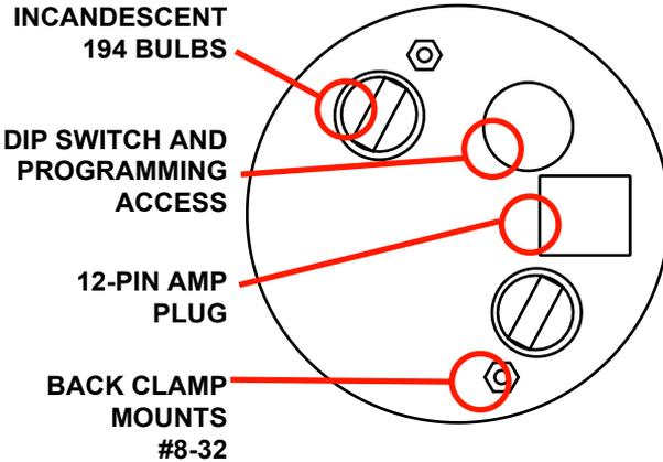
The features are shown at right. To access the DIP switches, remove the rubber plug.
