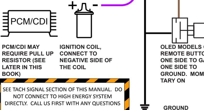
SEE TACH SIGNAL SECTION OF THIS MANUAL. DO NOT CONNECT TO HIGH ENERGY SYSTEM DIRECTLY. CALL US FIRST WITH ANY QUESTIONS
