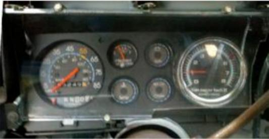
Remove lens/plate and original gauges (not re-used)
