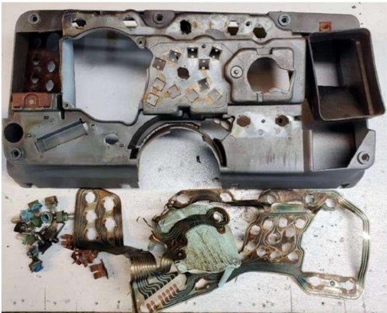
Remove the printed circuit ribbon. If its in bad shape, do not worry as it will not be used in the new installation.
