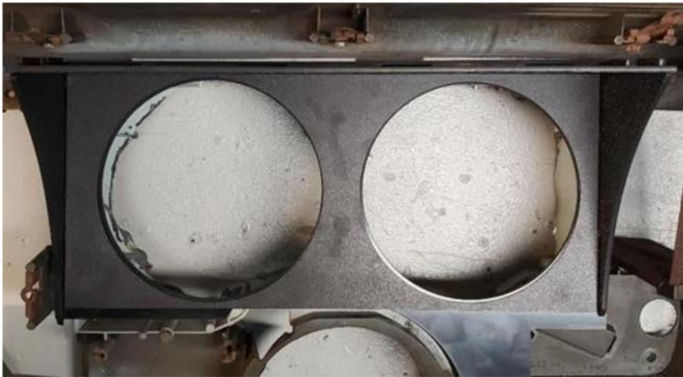
Set the bracket in place and mark with a marker where to trim.
