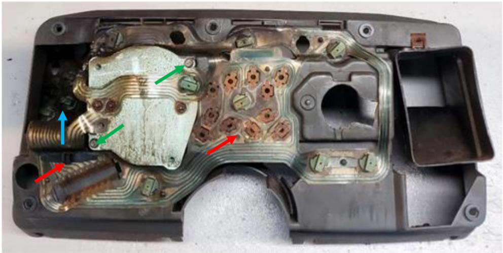
To remove the original flexible circuit, start by unscrewing the plate on the left (green arrow) (2 screws) and removing all bulb sockets, including the sockets on the indicator panel (blue arrow).
