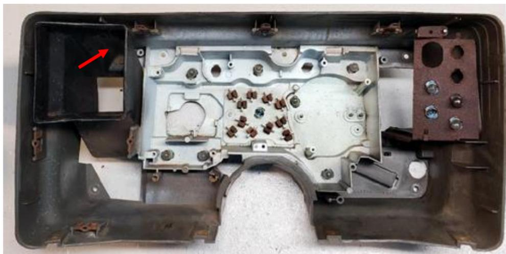
Housing will look like this. Remove left HVAC vent by removing single screw shown.
