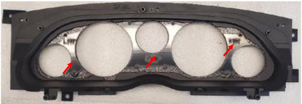
Place the top panel in the bracket/spacers/shroud assembly. Align the factory shroud holes to the main bracket and secure with original screws or #6 self-tapping (red arrows).
