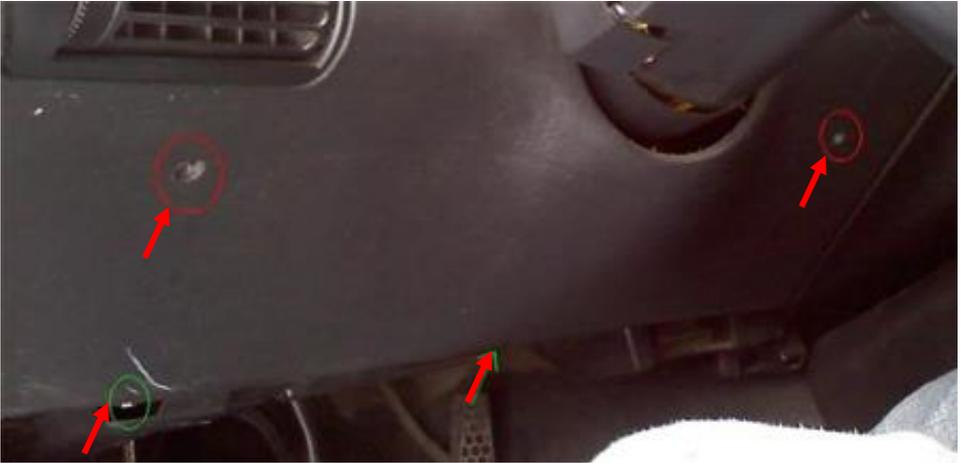
Remove the radio cover piece with the 5 8mm screws shown here. The cover then can be pulled off.
