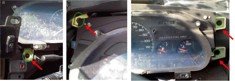
Disconnect the cluster plug on the left rear side and the cluster should pull out of the dash.
