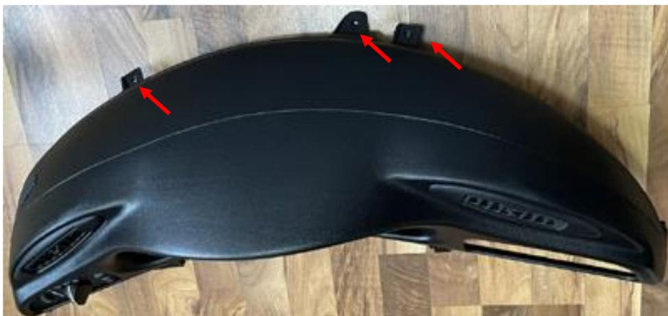
Remove the fasteners on the lower left portion of the trim bezel.
