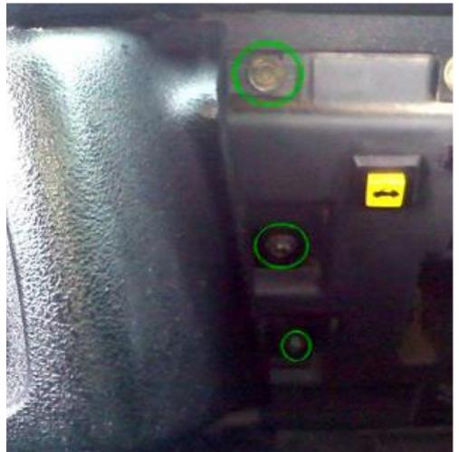
Remove the driver side A-Pillar. Pry away and there are 3 tabs holding it in place. You must have the door open.
