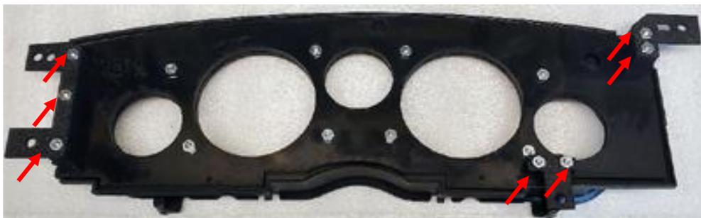
Test fit panel and make any adjustments. Make sure there is clearance in the back for the gauges and wiring. Remove any material to allow the gauges to be set back in place.
