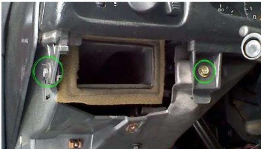
Remove this fastener on the right side of the dash bezel. Lower the tilt column if you have not done so already and remove the trim piece.
