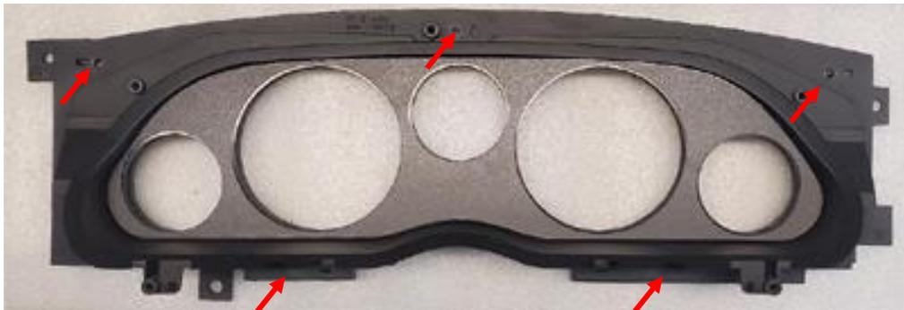
Fasten the top cover to the main bracket using the 8-32 nuts and lock washers you removed earlier.
