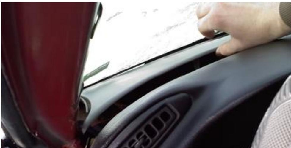
Remove the 7mm screws holding the top under the dash pad.
