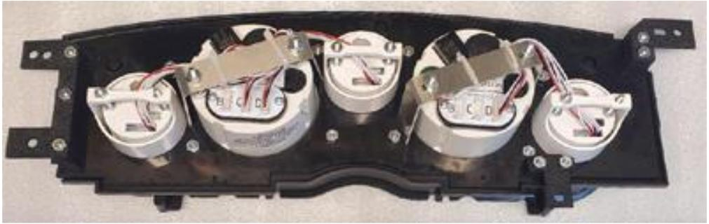
Remove the test fit assembly. Wire according to the gauge wiring booklet. We recommend a good vehicle diagram from a repair manual in addition to probing the wires to verify connections.
