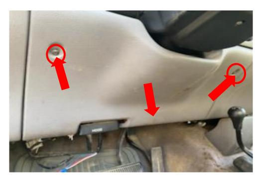
STEP 8: Reinstall bezel and bolt the column back together with the original bolts. Now its time replace the lower panel and screws.
