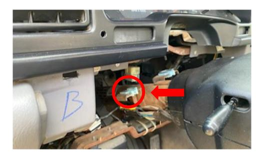
STEP 4: Drop Column out of the way and rest on seat. Disconnect the gear shift indicator from the column.
