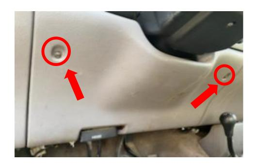
STEP 2: Remove lower dash panel screws and remove panel by pulling downward
