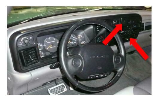
STEP 1: Remove the cup holder and ashtray by pulling them out and removing the two screws from both items.
