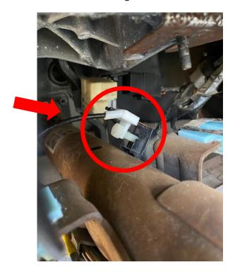
STEP 8: Place the column shifter into park, at this point check and make sure the indicator is adjusted correctly. If not, use this to adjust the indicator.
