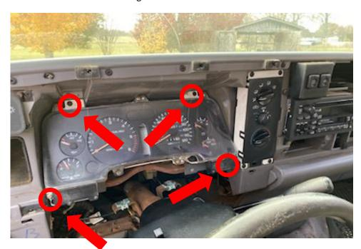
STEP 5:Remove gauge bezel by carefully prying back from the top Next you will remove the four screws holding the gauges in. Disconnect all harnesses and remove the old cluster.
