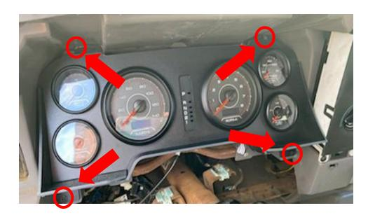
STEP 7: Reinstall your direct fit bracket into the factory mounting location with the original screws.
