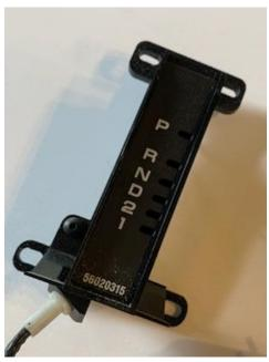
STEP 6: Carefully remove the new indicator from the NVU bracket. Now carefully pull your old shift indicator from your old cluster.
