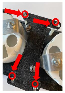
Reinstall the gear shift indicator to the new direct fit bracket
