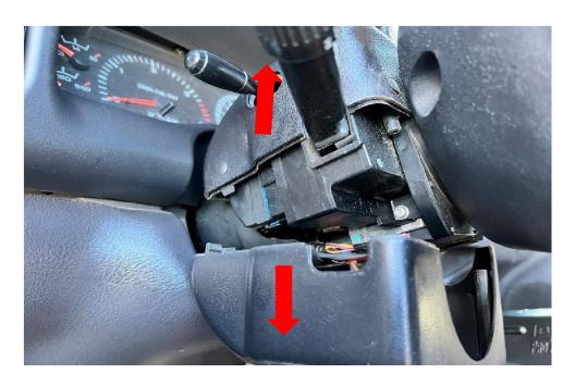
STEP 4: Remove top and bottom steering column covers.
