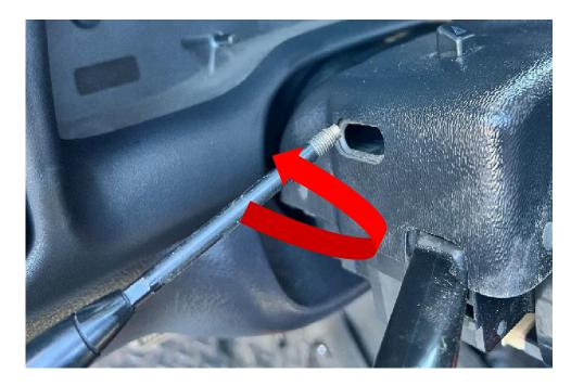
STEP 2: Remove steering wheel tilt arm by turning counterclockwise
