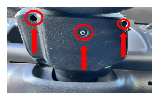
STEP 3: Remove the 3 T20 Screws from the bottom steering column cover.
