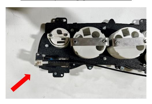
Step 13: Install shift indicator onto back of new cluster.
