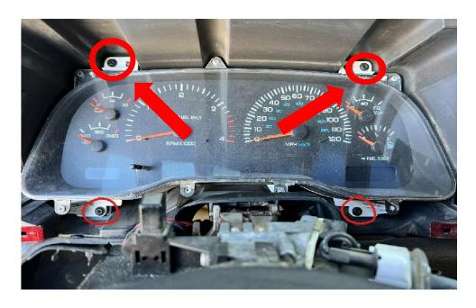
STEP 6: Remove 4 screws from cluster assembly.
