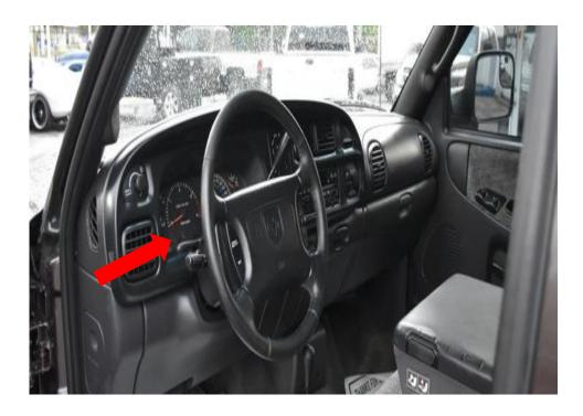
STEP 1: Tilt steering wheel to the lowest position.
