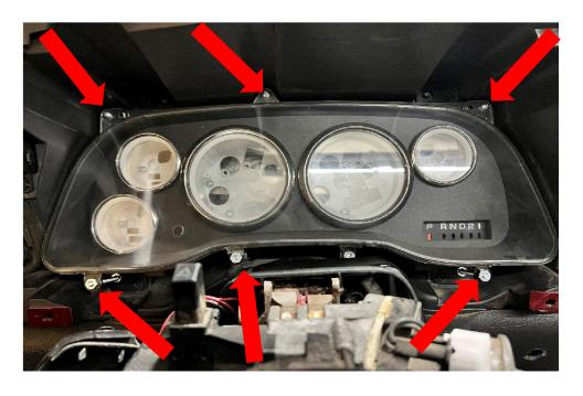
STEP 14: Install new cluster into dash reusing original cluster mounting screws.
