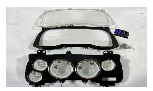
STEP 12: Assemble plastic covers onto new gauge cluster with supplied hardware.
