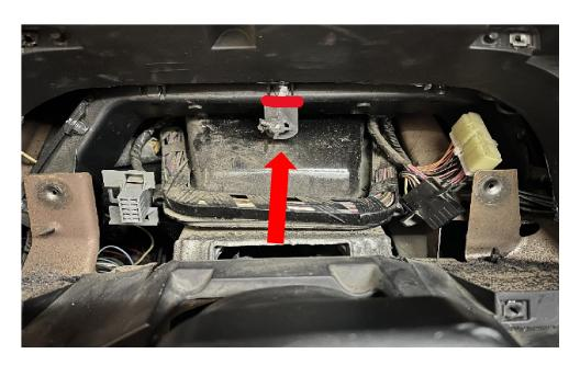
STEP 10: After removing plastic panel cut on red line in picture removing plastic support.
