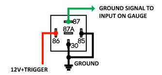
To trigger NVU indicator lights (in the gauge) will require 12V+ to illuminate the LEDs. If your signal is a ground trigger (brake light for example) there are 2 methods:
