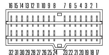
This plug does not have an "UP" or "DOWN" locator. To plug in properly, cable tie slot must be aligned with locators on plug where the spacing of the pins has a gap.
