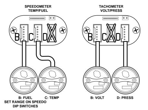
The B, C and D pins are used to connect the 2-1/16" gauges through the master gauge. All functions and lighting are done through this plug. Refer to the wiring diagram for each kit for proper wiring. Below is each plug's function and its corresponding input wire color. Pins C and D are the same on the speedo and tach.
